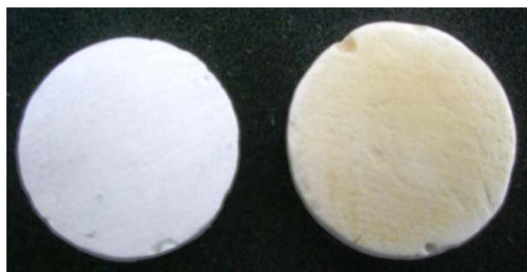
Figure 2. Photographic images of PolyHIPE Polymer discs before (left) and after transformation to an anion exchanger (right). [Color figure can be viewed in the online issue, which is available at wileyonlinelibrary.com.]
